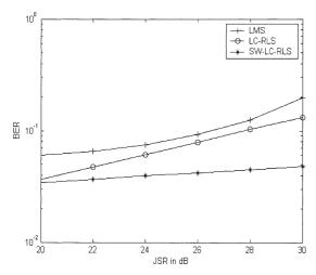
**Fig.4** Performance comparison of BER against joined JSR for RAKE receivers combined with different adaptive multiuser detectors under 3-paths fading channel.
