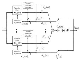
Fig. 1 General block diagram of the adaptive multiuser RAKE detector.
