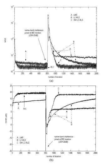
**Fig. 2** Learning curves comparison with different techniques under fading channel with a narrowband interference JSR=20 dB (a) MSE (b) output SINR.
